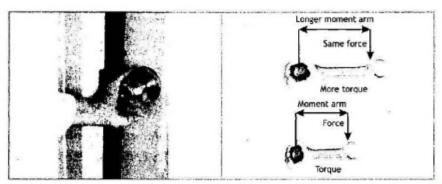
A door handle is fixed at the outer edge of the door so that it opens easily. A larger force would be required if the handle were fixed near the inner edge close to the hinge. Similarly, it is easier to tighten or loosen a nut with a long spanner as compared to a short one.
