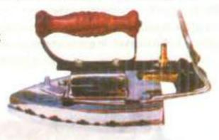
is put at on', the lid is lifted and the burner is lit. The lid is then closed and the iron is allowed to get hot. The flame can be adjusted by moving the knob or regulator fixed with the connection.
