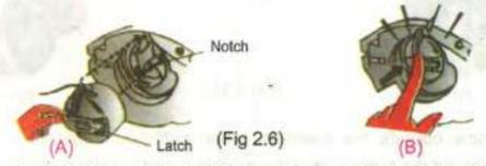
the little finger in the bobbin case is opposite to the notch at the top of the shuttle case. (Fig 2.6A)
