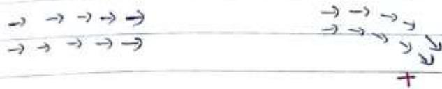
In electric field, rays deflect towards positive plate which proves Cathode rays is a beam of negatively charged particle.
